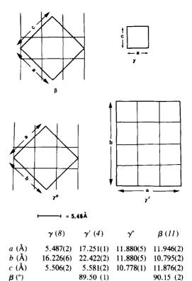
Fig. 1. Correspondence between elementary cells (direct cells) of  $\beta$ ,  $\gamma$ ,  $\gamma'$ , and  $\gamma''$ .
